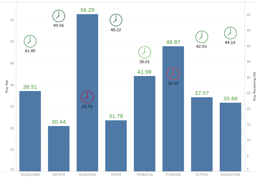
Figure 4: Pipe Average Pipe Age and Remaining Life of Each Scheme*
