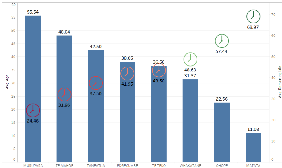
Figure 6: Manhole Average Pipe Age and Remain Life of Each Scheme*
